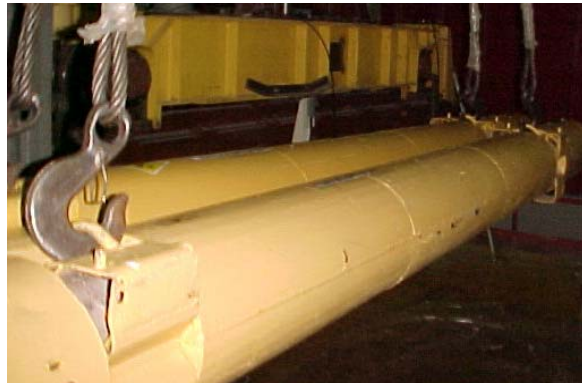
Transportation of an FA to the warehouse
