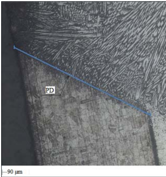
Figure 1 Example of the photo depicting a microsection of the fuel element welded joint with the depth of the weld penetration measured
