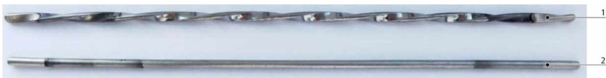
Figure 1 — Typical appearance of pre-test specimens: 1 — cylindrical specimen; 2 — twisted pattern
