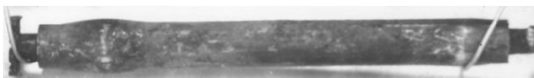
Figure 3 - Appearance of the irradiated model with cladding from 42KhNM alloy
