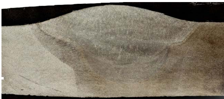
Figure 2. Welded joint macrostructure for the OPG-1 shell.
